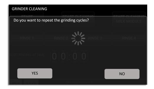
Refill cleaning device if "YES" button in previous step. If press "NO" button skip to "Insert bean hopper" next step.
