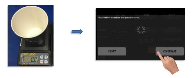
4) A predefined grinding time will be activated. Collect all grounded coffee and weight it.
