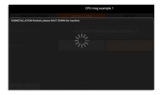
At the end of the uninstall cycle, the boiler water temperatures will be set to zero and the VM set automatically "first installation" parameter to zero.
