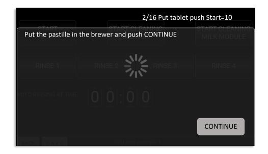
Insert a cleaning tablet and tap on CONTINUE. The Variflex will move up to close the infusion chamber. While Variflex moves on place, "wait please" will be displayed on screen.
