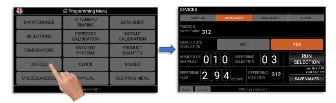
To modify the Varigring reference position "ENABLE AUTO REGULATION" option should be temporary disabled (set on 'NO').
