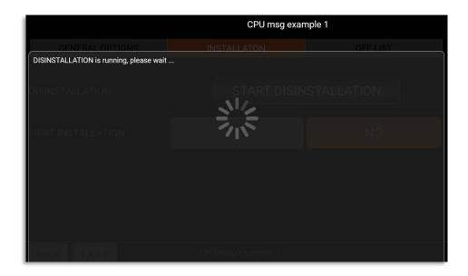
"FIRST INSTALLATION" parameters automatically set to zero to avoid that VM warm up without water in hydraulic circuit. First installation procedure starts during next VM reboot (look at "6.8.1 FIRST INSTALLATION PROCEDURE").
