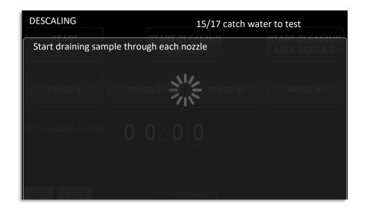
Check the pH of collected sample. Tap on "CONTINUE" button to continue or "REPEAT" button to repeat the previous steps to clean properly the hydraulic circuit.
