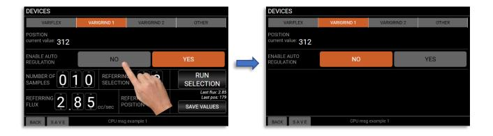
Save (tapping on button "SAVE"). Move to "ESPRESSO CALIBRATION" section.
