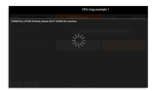
Shut down the VM at the end of the uninstall cycle. The VM set automatically "first installation" parameter to zero: first installation will execute during next VM reboot to fill water circuit.
