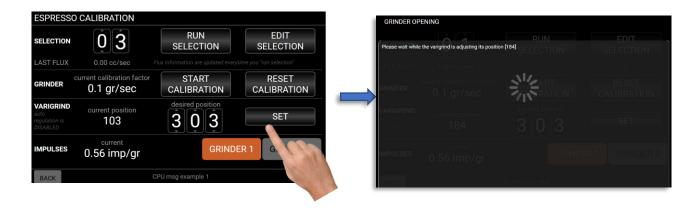
Varigrind will reach required position, as shown in "current position" value.
