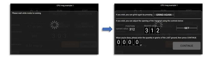
Reach a desired weight (as an example 20.5g), insert the value in its screen box, then tap on "CONTINUE" button.
