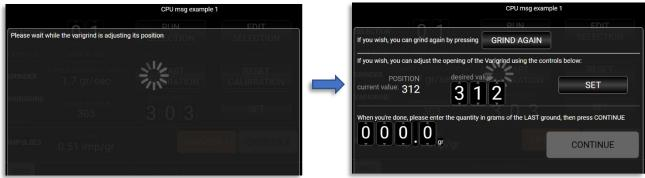
Varigrind motor will move to the new position. The message "Please wait while the Varigrind is adjusting its position ['x']" reports Varigrind is moving to desired position. The updated value for current Varigrind engine position will be 'x'.
